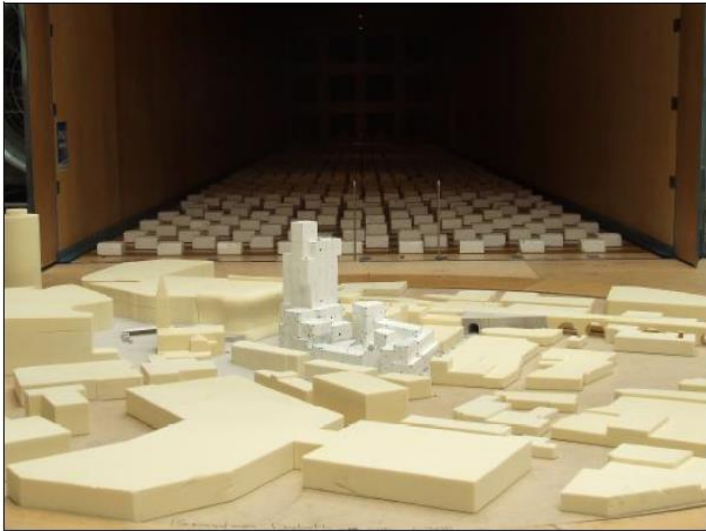
Figure 15.5: Wind tunnel test model (RWDI 2008 3 ).
